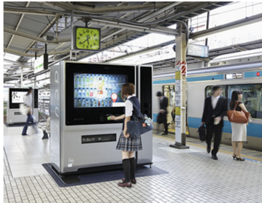
Figure 1: A vending machine used for the experiment on a train platform: A camera at the top of the machine recognizes the customer's age and gender, and the machine makes recommendations based on the observed consumer characteristics. The image is supplied by the company.
